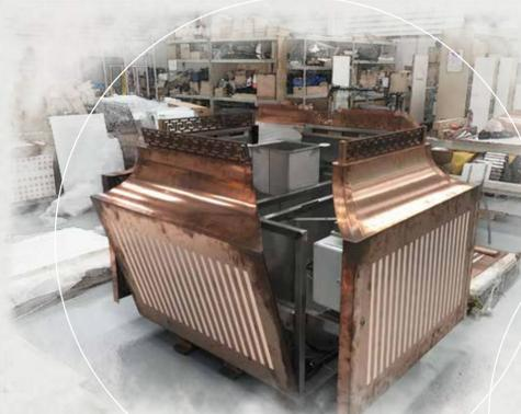
The tree planter opens to receive the tree pre-planted and guyed in a stainless steel liner
